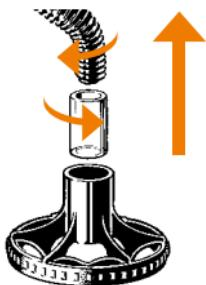
*Pull the Cooling Coil out of the Filling Chamber Cap*
