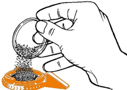
Always fill the Filling Chamber completely up to the upper edge
