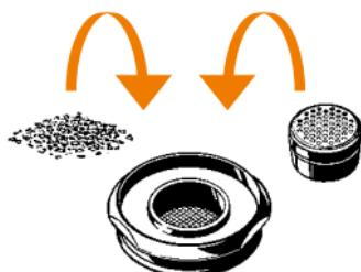
*Fill the Filling Chamber Reducer with ground plant material directly or with a filled Dosing Capsule*
